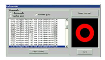
When creating a custom component, you may find that the pad you need is not in our pad library. In this case, press the *Create new pad* button in the Pad Manager to define a new pad size. Here you can create a new *via*, *through-hole* or *surface-mount* pad. When designing a pad with a through-hole, the pad diameter must be at least 0.017" greater than the diameter of the hole.
