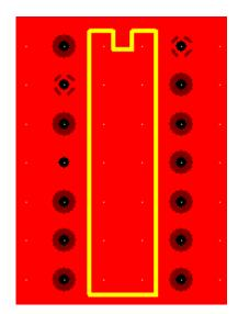
To look at the actual inner layer planes, open the *Options* dialog box and check either *View Power inner layer* or *View Ground inner layer*. Here we show what the *Power layer* looks like for the example above.
