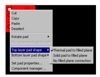
Pads inside a plane can be connected to it using either a *Solid* or *Thermal* pad shape.
